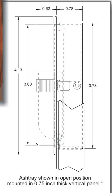
Ashtray shown in open position mounted in 0.75 inch thick vertical panel.\*
