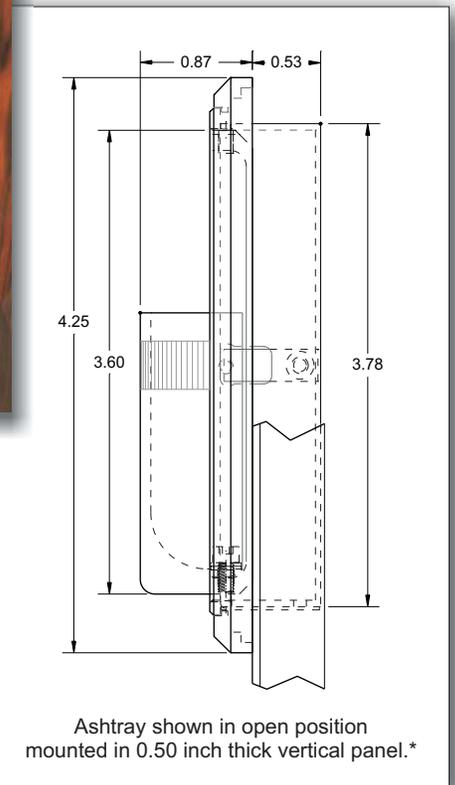
Ashtray shown in open position mounted in 0.50 inch thick vertical panel.\*
